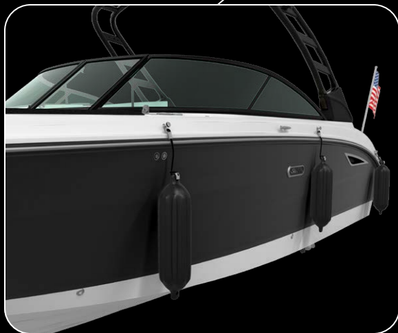
Quick connect fender clips
